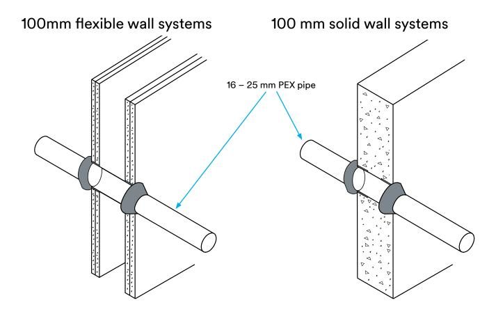
To view all current 3M Fire Protection Approvals please visit www.3M.com.au/fireprotection See Regulatory Information Report (RIR) # 4539800.1 for 3M<sup>™</sup> Fire Barrier Watertight Sealant 3000 WT. \*3rd Party Fire Testing to AS 1530.4 & AS 4072.1 completed.
